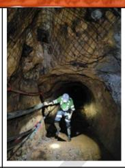
The cables not only provide necessary connection but are used as a guide to find the way out if helmet lights fail. Cables right hand to find the exit.
