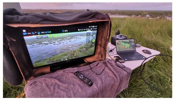
Viewing live drone footage of a target wetland. Heat signatures can be investigated if they appear to be related to the target species, such as bittern or harrier. The towel and blanket help reduce glare on the screen. Credit: Henry Caley.
