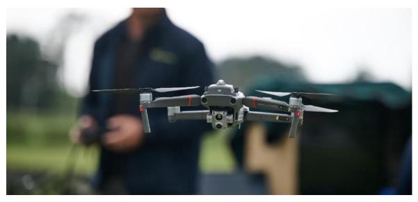
Drone being piloted with a hand-held controller. The drone carries thermal and visual light cameras, weighs around 900g, and can reach 72km/h. Credit: Craig McKenzie.
