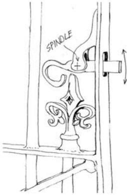
Figure 26. Sketch showing detail of door latch operation.
