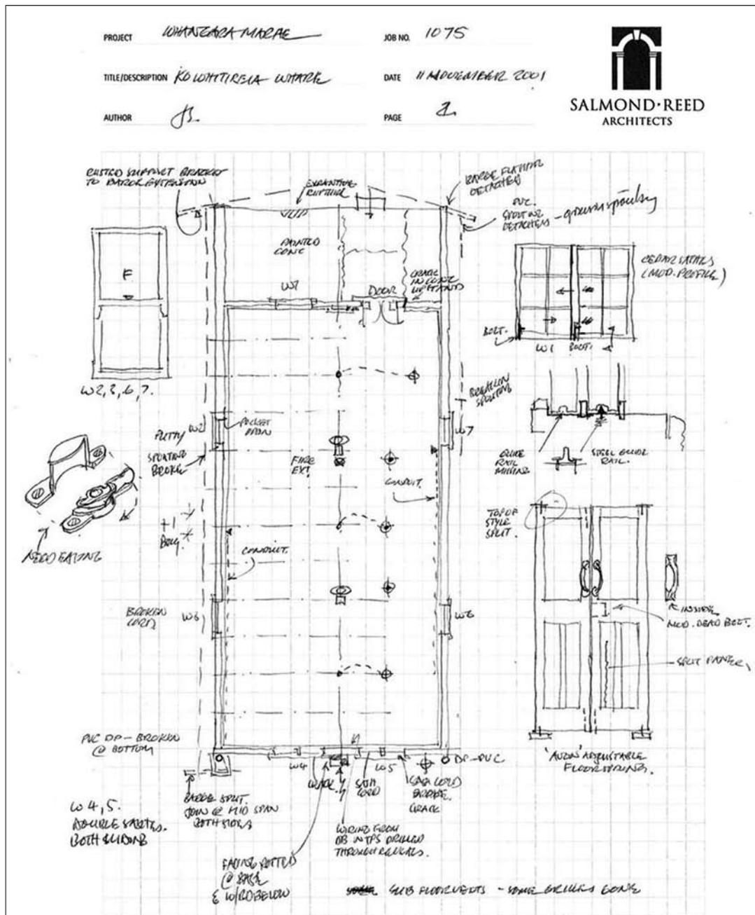
Figure 25. Site sketch plan for church at Whangara, near Gisborne, showing showing some construction details and recording the condition of various features.
