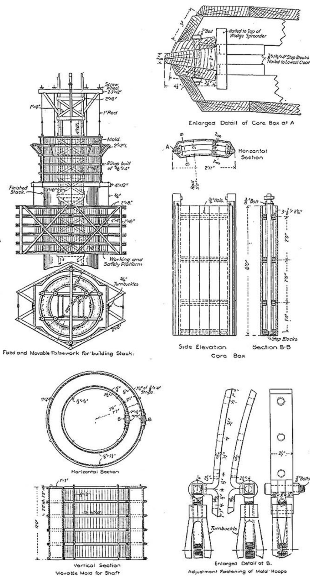
Figure 6. Shuttering and moulds used by Ransome's in 1903 for a reinforced chimney 165 feet high (from Marsh 1905).
