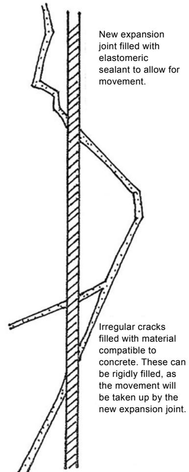
Figure 21. Insertion of an expansion joint to repair irregular active cracking.
