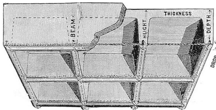
Figure 5. Ransome's system, which was widely used in the USA in the early 1900s, was similar to the Hennebique system, except for the use of square twisted reinforcing bars (from Marsh 1905).
