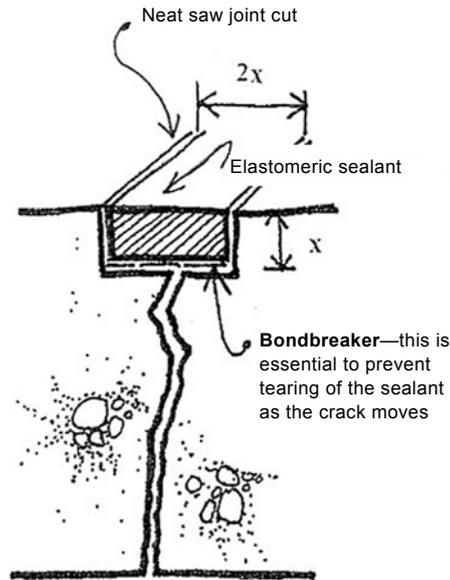
Figure 20. Repair of an active crack.
