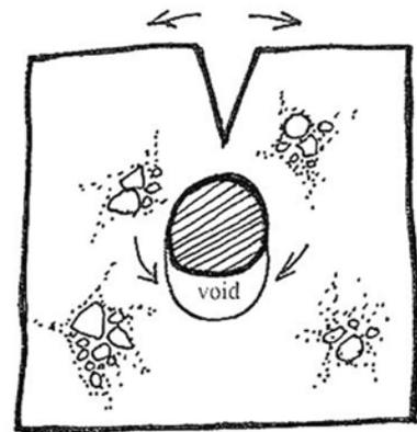
Figure 16. Typical settlement crack.
