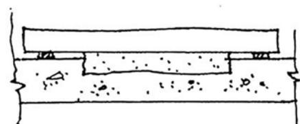
**Correct method of finishing**—the strike off board is held slightly above the level of the concrete. A thorough curing process should follow to prevent shrinkage cracking.
