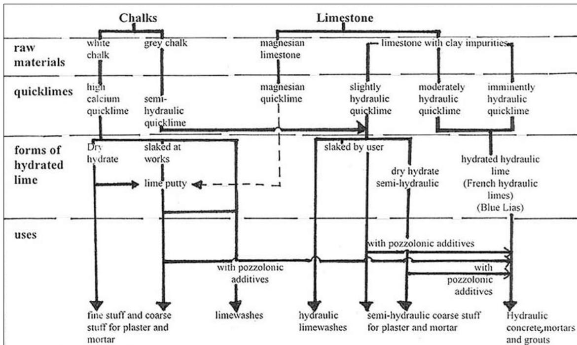
Figure 11. Types and uses of lime (from Cowper 1927).
