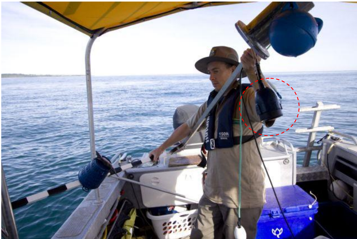
Figure 18. BRUV setup prior to deployment. Red circle denotes Splashcam® drop camera. The drop camera is used to assess substratum suitability at the start of the deployment.
