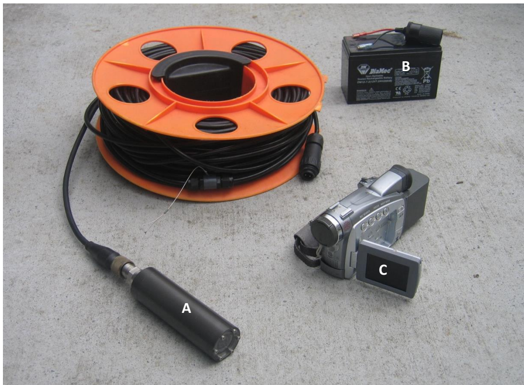
Figure 19. Drop camera equipment: A) MDEL drop camera and 70m coaxial cable; B) 12 V rechargeable battery pack used to power the drop camera unit; and, C) Digital video recorder with movable screen. This setup is used for real time substratum and habitat assessment. All components are linked together in a customized waterproof case (not shown). Note: the video recorder is powered by a long-life (8h) 7.4v battery pack specific to the video recorder.
