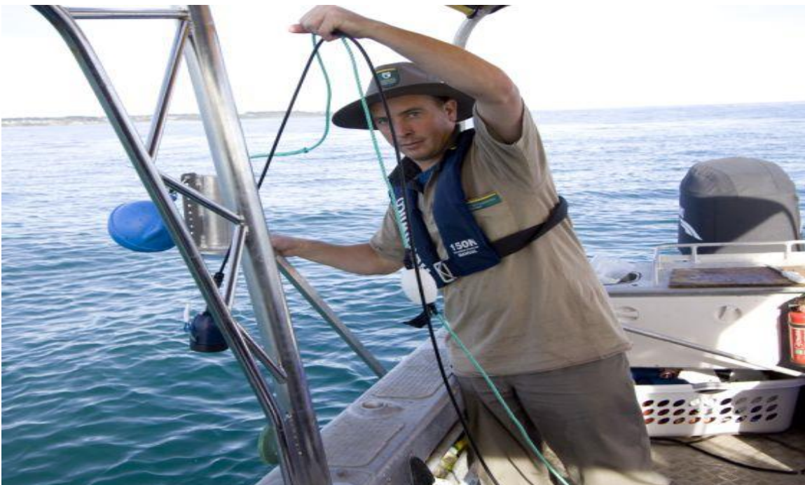
Figure 25. Immediately prior to deployment. Note: the BRUV coaxial cord (black) plus surface rope (green) and buoy (not in field of view) are held together by the surveyor to reduce the chance of entanglement.
