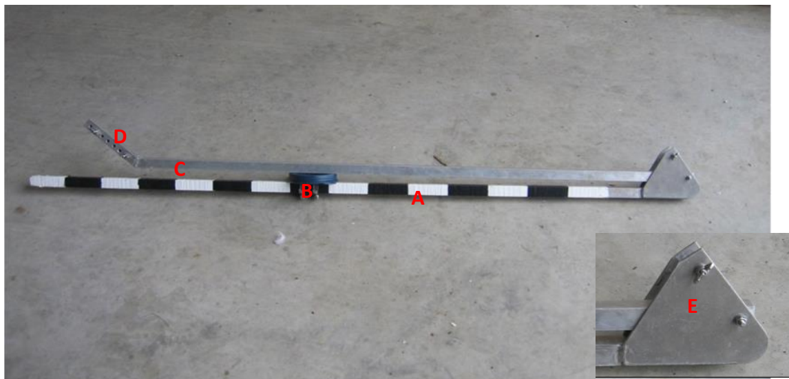
Figure 16. BRUV frame in folded position with housing removed. A: Bottom scale bar B: base of bait pot; C: moveable angle bar; D: housing attachment section and associated drill holes used to attach to the housing; E: 10mm thick polycarbonate lens.
