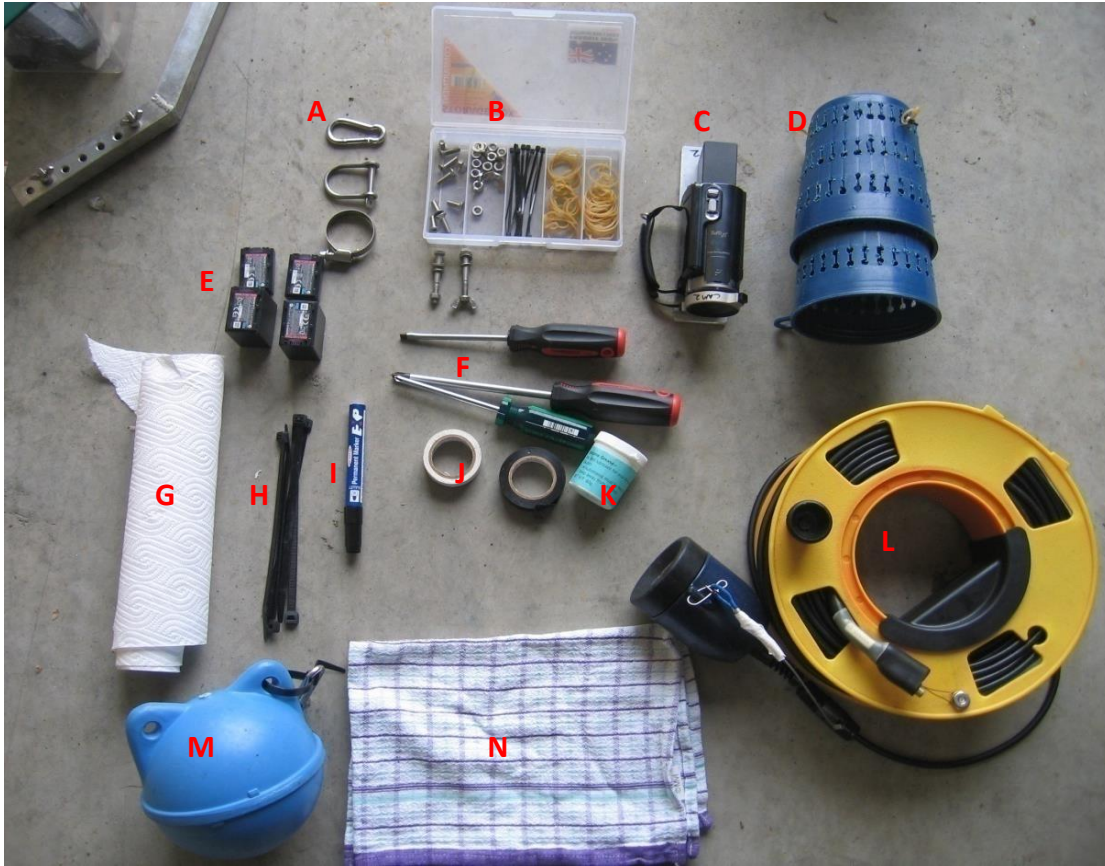
Figure 20. Typical hardware and consumables required for undertaking a BRUV survey. A – Fasteners (shackles, carabinas and hose clamps); B – Rubber bands, cable ties and spare screws; C – Digital video camera; D – Bait pots; E – Rechargeable video camera batteries; F– screwdrivers; G – Paper Towels; H – Cable ties; I – Permanent marker pen; J – Electrical tape; K –Silicon grease; L – Drop camera; M – Pressure Buoy; N– Cloth; O – Silica gel; P – Fuses. Hardware aside, include a spare of every item.
