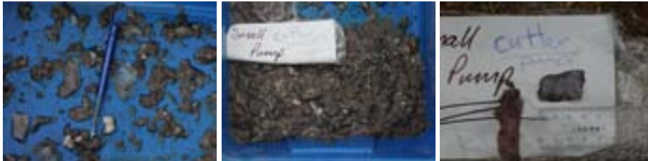
Figure 2: Photographs of fish waste after being processed through (a) the hasher, and (b) the hasher and the cutter pump.
