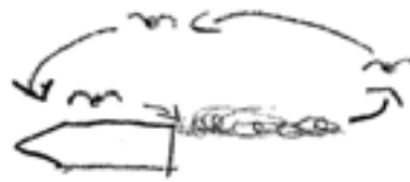
Figure 9: Observer sketches of the different discharges from (a) the hasher pump (Trip B, tow 19) and (b) the cutter pump (Trip B, tow 67). The hasher pump discharged in pulses, whereas the cutter pump produced a continuous discharge.
