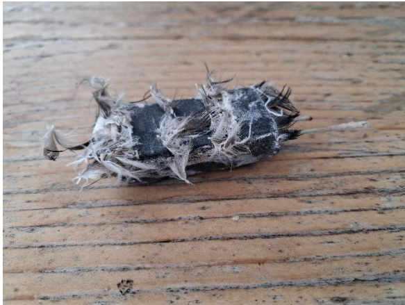
Figure 4. Recovered device found on the edge of breeding colony. Showing the underside of the device, and how the tape has remained attached to the device, but some feathers have become unstuck, and others preened out by the bird.
