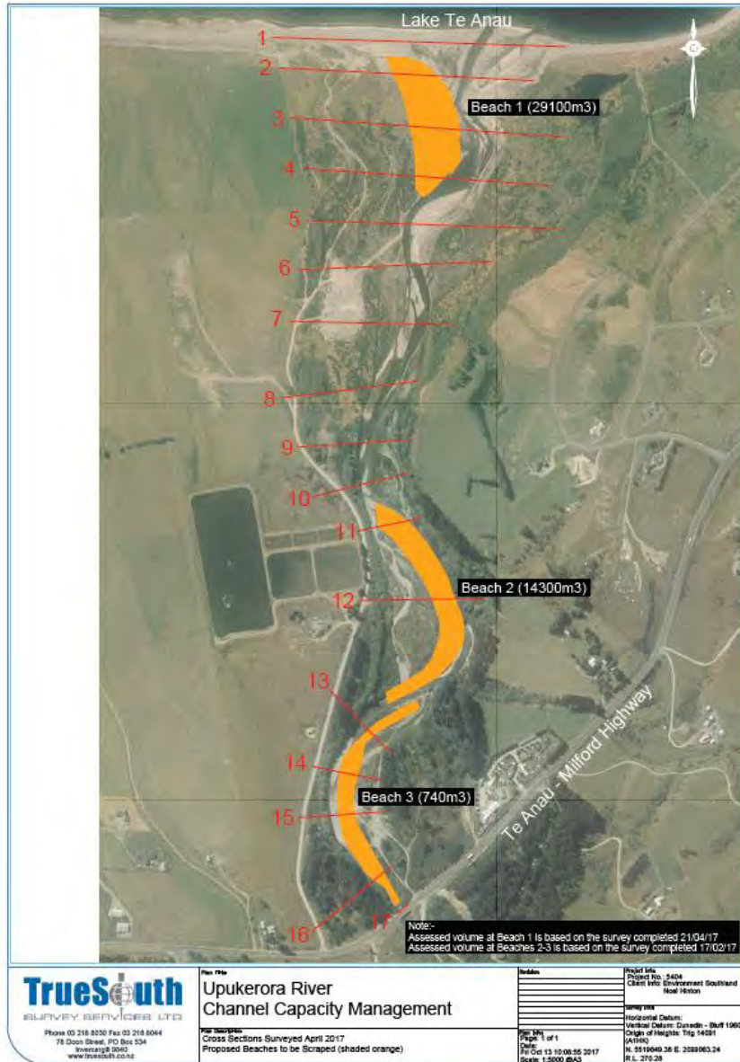
Figure 3. Plans showing details of proposed gravel extraction site along the Marakura/Upukerora River, Te Anau. The orange polygons indicate the three sites of gravel extraction (Source: Client Supplied Image).
