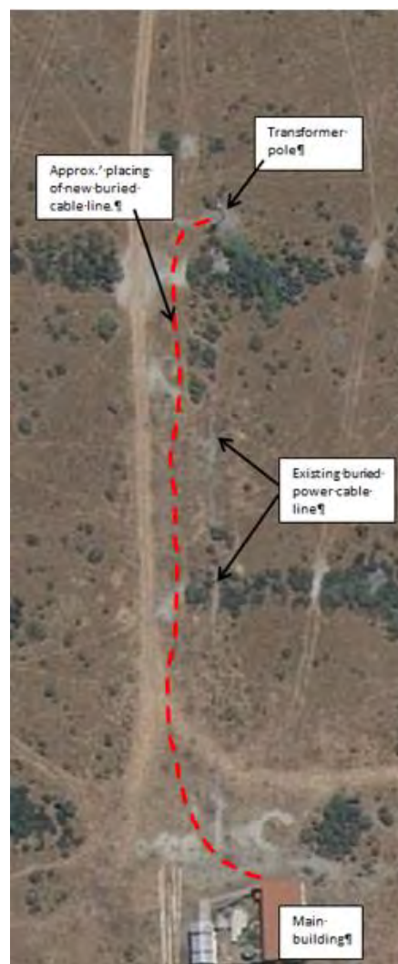
Proposed location for placement of new power cable
