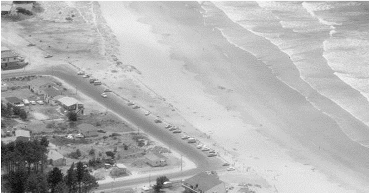
Figure 9: View of Esplanade Drive in 1979, showing dune width remaining after 1978 storm. The shoreline has not been this far landward since.
