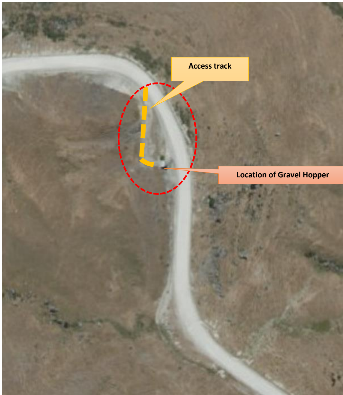
Figure 18: Location of Gravel Hopper incl access track
