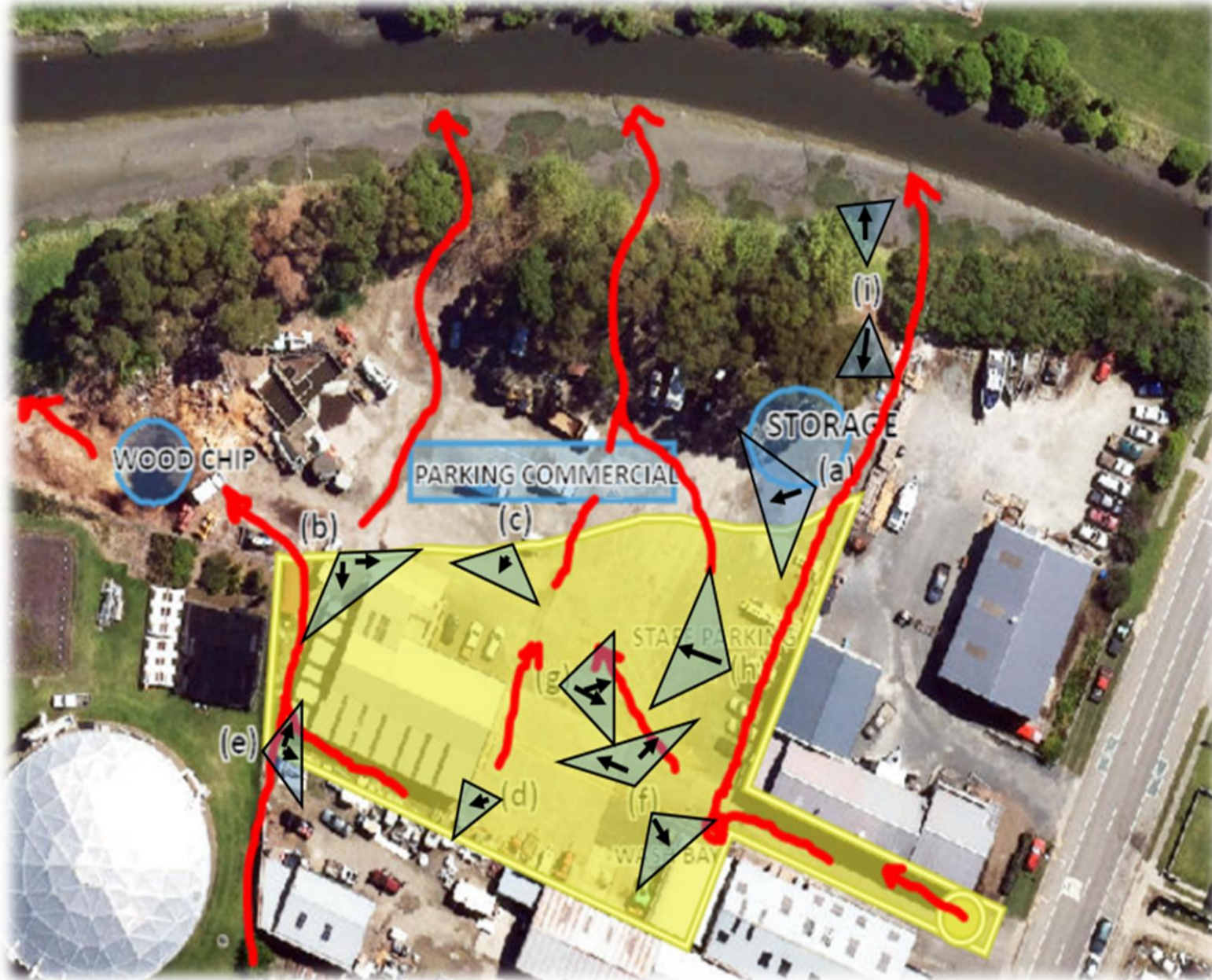
Image 3.3: Provides - Red lines Stormwater runoff | Yellow is the fenceline boundary | the triangle provide photo points and the direction photos taken.
