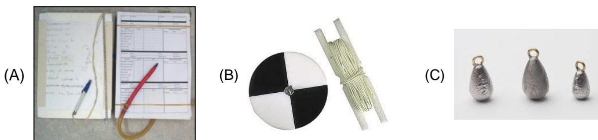
Figure 2. A selection of resources required to measure Secchi depth: (A) datasheets (on waterproof paper), clipboard and pencil; (B) Secchi disk and measuring line; and (C) weights, needed when sampling in high-flow areas.
