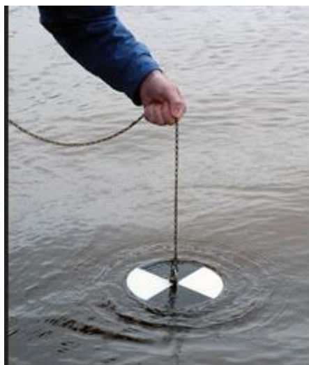
Figure 9. The Secchi disk and measuring line slowly lowered over the side of the boat.
