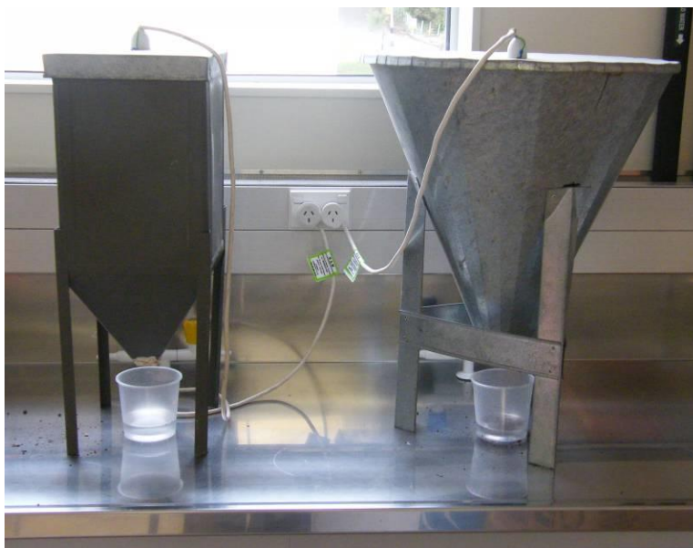
Figure 5. Two different designs of Tullgren funnel. Both have light bulbs in the lid (Fig. 6) which progressively dry material suspended on coarse mesh inside (Fig. 7). Invertebrates move downward as the material dries and fall into the collecting containers below.
