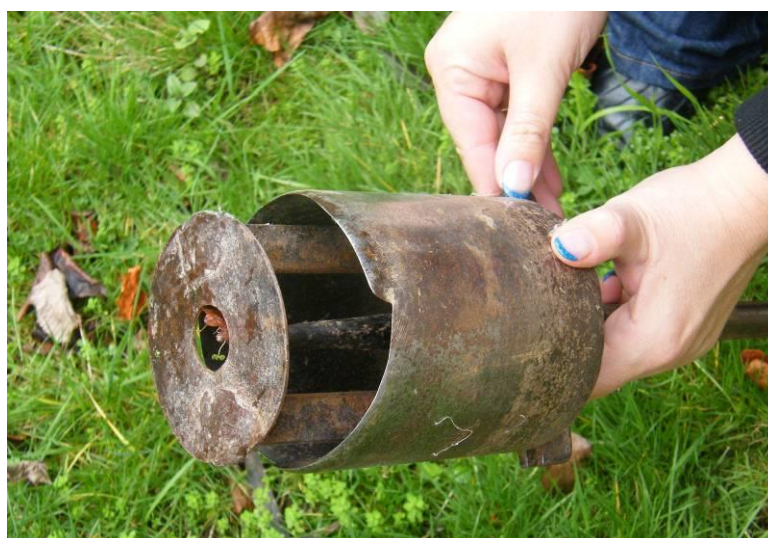
Figure 4. End of a soil core sampler. The notch in the cylinder helps dig the instrument into the soil when it is twisted while the disc (attached to the yoke shown in Fig. 3) is used to push the sample out of the corer.
