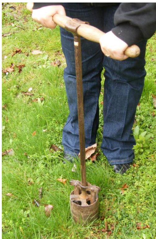
Figure 3. Soil core sampler. The handle is used to push and twist the corer into the soil. Near the base of the handle is a yoke attached to an internal disc (shown in Fig. 4) which is used to push the soil sample out afterwards.
