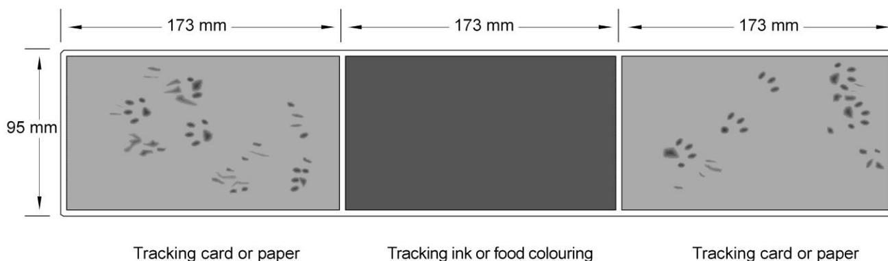
Figure 3. Tracking tunnel tray showing paper/card and tracking ink tray/panel dimensions.
