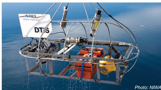
Special equipment is needed to survey the deep seabed. DTIS is equipped with high-definition video and still cameras, floodlights and a depth sensor. Towed behind a research vessel, DTIS relays a live stream of underwater footage to the vessel above.
