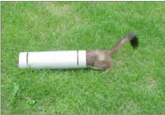
Stoat entering PVC tube with adhesive gel on a rubber band stretched across the aperture, designed for hair collection.
