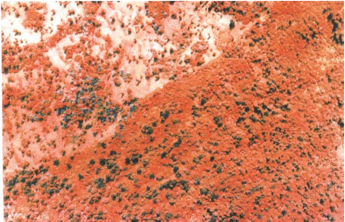
Figure 1. A typical colour-infrared (CIR) scene, showing forest in darker red tones and pasture in the lightest red tones. Blue/grey tones are dead vegetation. Olive green tones are rimu ( Dacrydium cupressinum ).
