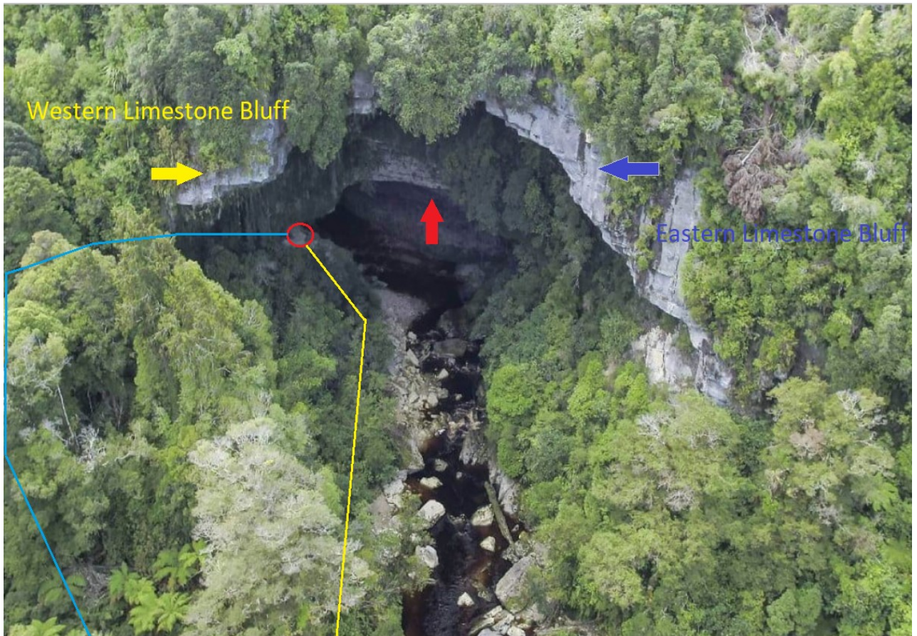
Photograph 1: General view of the Oparara Arch Complex from the south. The Natural Bridge feature (blue arrow) is located in front of the southern portal of the main arch (red arrow). The existing track is shown as a yellow line and the proposed track realignment is shown as a blue line. An overhanging area exists (yellow arrow) above the proposed track and is attached to the bridge feature, and southern portal of the arch feature. The existing viewpoint area (underneath the main arch) is shown by a red circle. Rockfall debris material can be observed within the active Oparara River channel. (Source-AirNewZealand)
