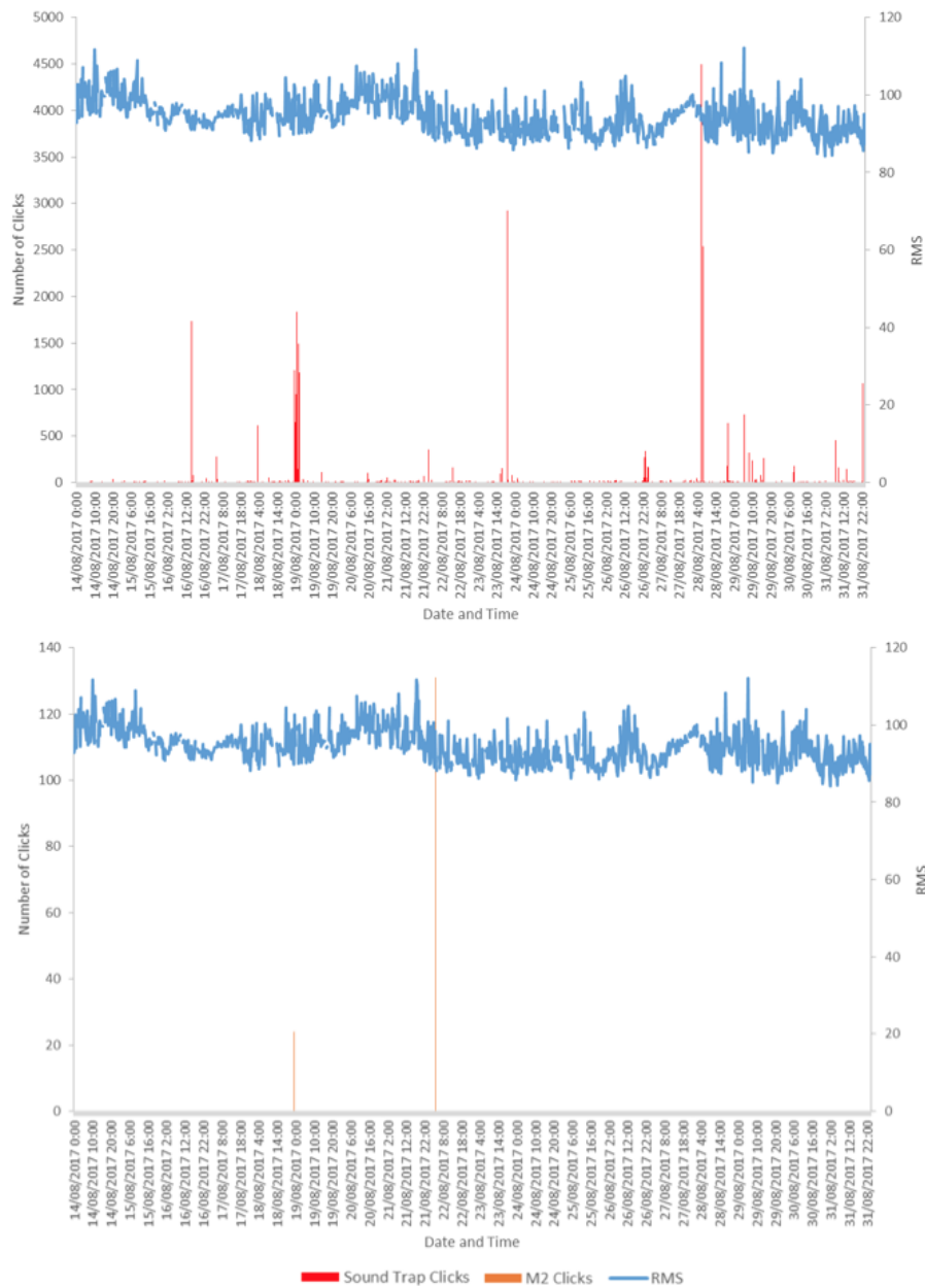
Fig. 13: Number of high quality NBHF clicks detected by C-POD M2 and the high frequency sound trap device, compared to the relative sound level represented as root mean squared (RMS) at mooring two from the 14/08/2017 at 00:00 to the 31/09/2017 at 24:00 NZST.
