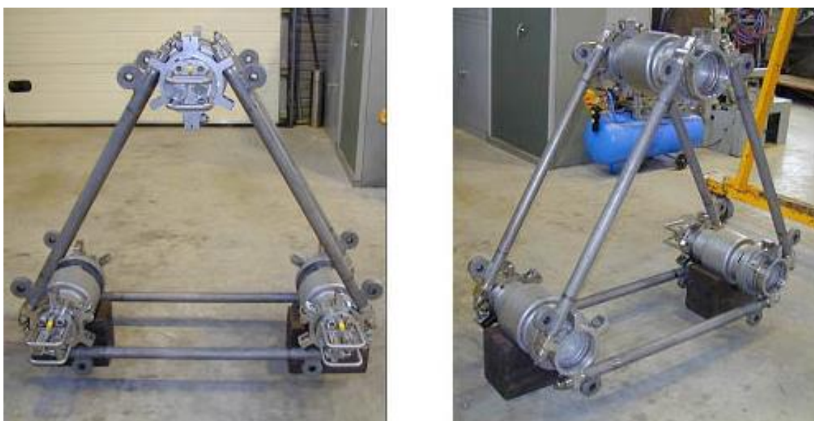
Figure 2 The 450 cubic inch triple G-Gun cluster inside standard Delta deployment frame (image courtesy of Schlumberger)
