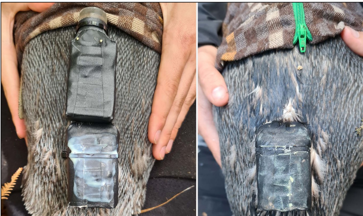
Figure 5. Combination of PenguCam video camera and AxyTrek GPS dive logger attached with tape to the lower back of a penguin (left) and after recovery of the camera the day after initial deployment. Groper Island, Bravo Group, Rakiura, 14 & 15 December 2020.
