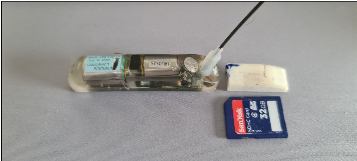
Figure 2. Wildlife Computers SPOT-275 satellite transmitter (left) and TechnoSmart Axy4 dive logger (right) that were deployed in combination to study hoiho foraging and dive behaviour in winter 2021; SD card shown for scale.
