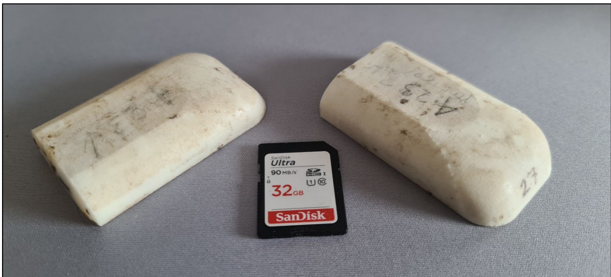
Figure 1. TechnoSmart Axy-Trek Marine GPS dive loggers used in this study; SD card shown for scale.
