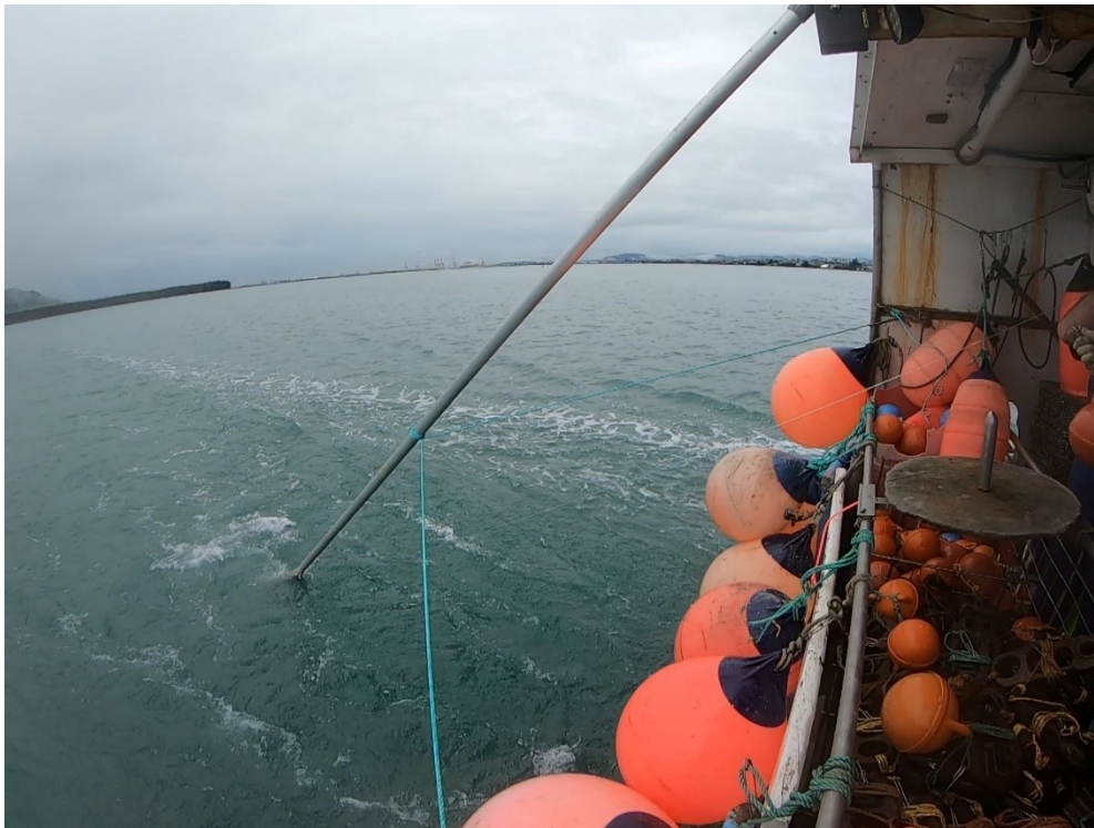
Figure 2d. Still taken from Go Pro camera mounted on the vessel showing depressor attachment and longline.
