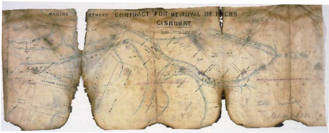
Fig 21: Surveyed chart of Turanganui River indicating rocks to be removed, Collection of Archives New Zealand Te Wbare Tobu Tubituibonga o Aotearoa
