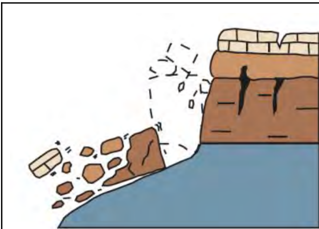
Figure 7. Schematic representation of a rockfall / topple 16 .
