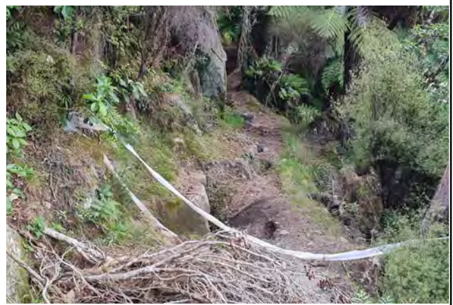
Figure 6. Translational slide with 0.5 m displacement along the bedrock/soil interface to the north of Tonga Quarry (Onetahuti Beach).
