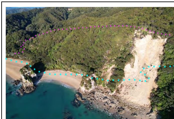
Figure 29. Newly constructed track (pink dashed line) located immediately upslope of the large landslide. Blue dashed line shows the approximate original track alignment.
