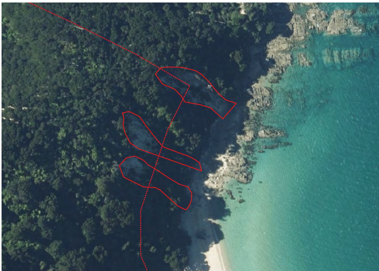
Item A1. Landslides visible in the 2022 aerial photo dataset at Skinner Point. The red dashed line shows the location of the track at the time of the event (the track has now been re-routed above the landslides).
