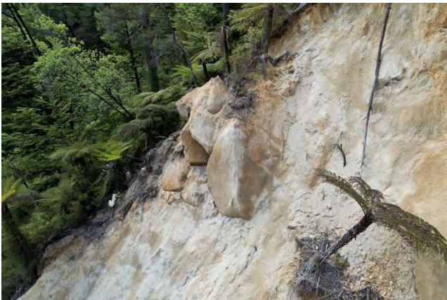
Figure 9. Granite corestones exposed in the upper part of the Torrent River landslide.
