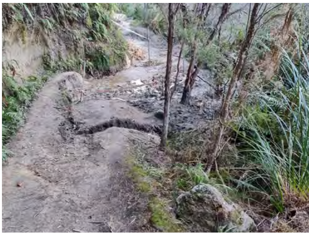
Figure 3. Translational slide with ~0.5 m displacement south of Tonga Quarry. It is likely that this landslide will continue to be active for some time.
