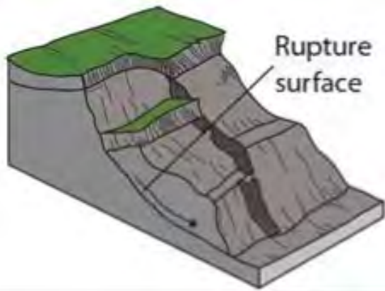
Figure 1. Schematic representation of a translational/rotational soil slide 12 .
