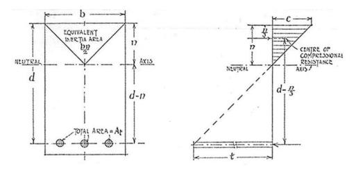
Figure 12. How a single reinforced beam resists compression and tension (from Jones 1913).
