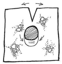
Figure 16. Typical settlement crack.
