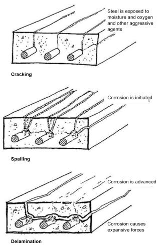
Figure 18. Progression from cracking to spalling to delamination in corroding reinforced concrete.
