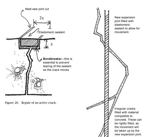
Figure 21. Insertion of an expansion joint to repair irregular active cracking.
