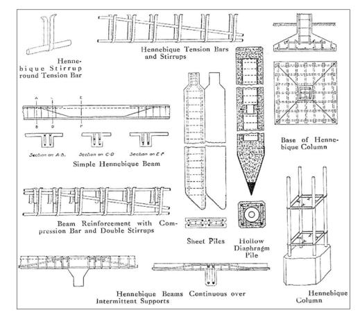
Figure 2. Hennebique system, showing general arrangement of reinforcement in beams (from Jones 1913).
