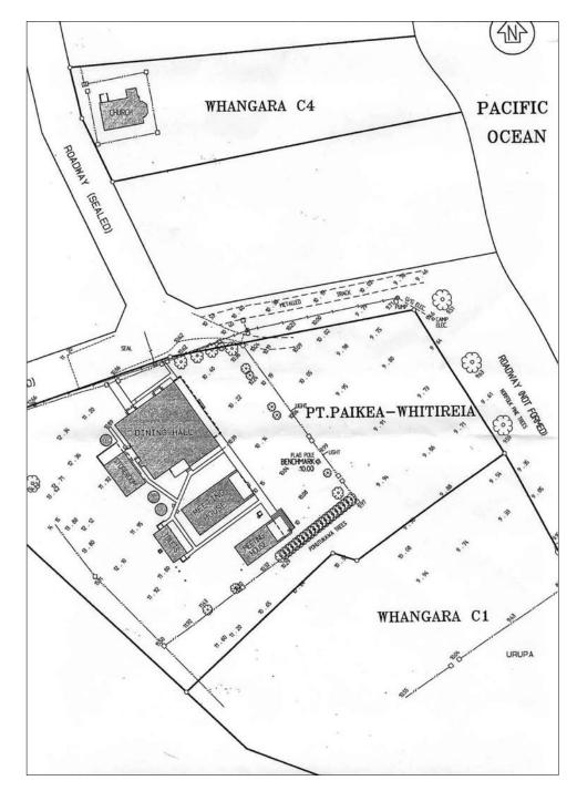
Figure 24. Surveyed site plan, showing key features, at Whangara Marae, near Gisborne (Grant & Cooke Ltd, Surveyors, Gisborne).
