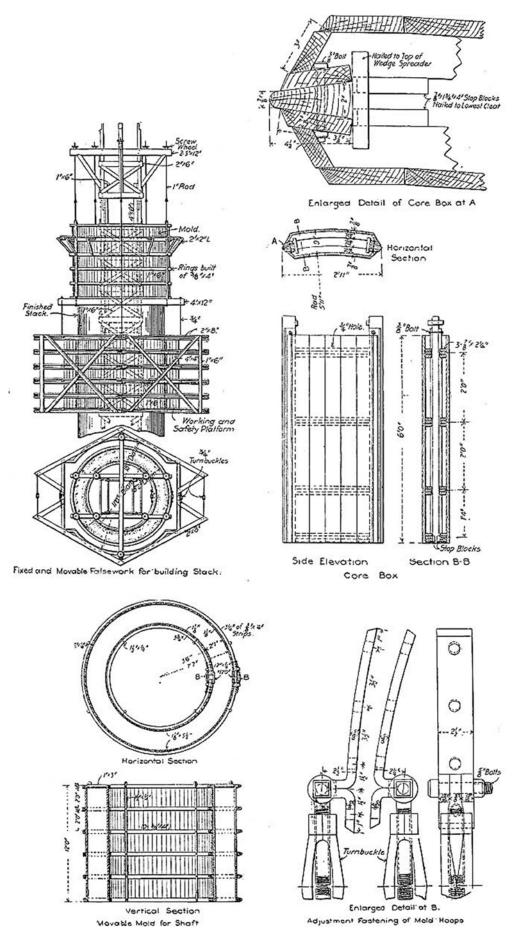
Figure 6. Shuttering and moulds used by Ransome's in 1903 for a reinforced chimney 165 feet high (from Marsh 1905).
