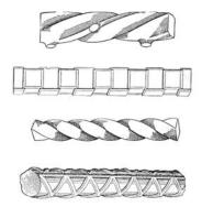
Figure 4. Examples of early steel bars designed to improve the bond between concrete and steel (from Kidder 1909).
