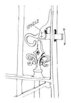
Figure 26. Sketch showing detail of door latch operation.
