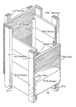
Figure 14. Typical column form with spiked-on front boards (from Jones 1913).
