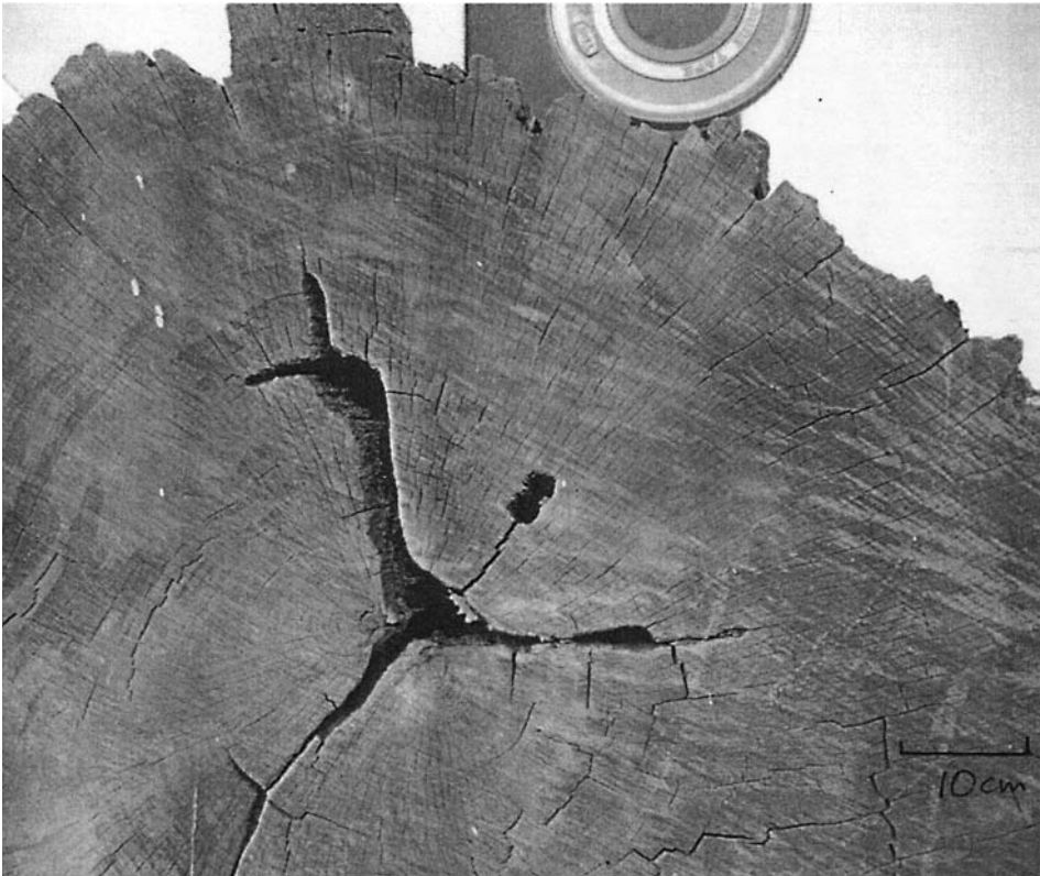
Fig. 7: Centre shake on kauri log in the Whitianga Museum. This would be indistinguishable from centre rot in an ultrasound scan. The shake is quite free from rot.
