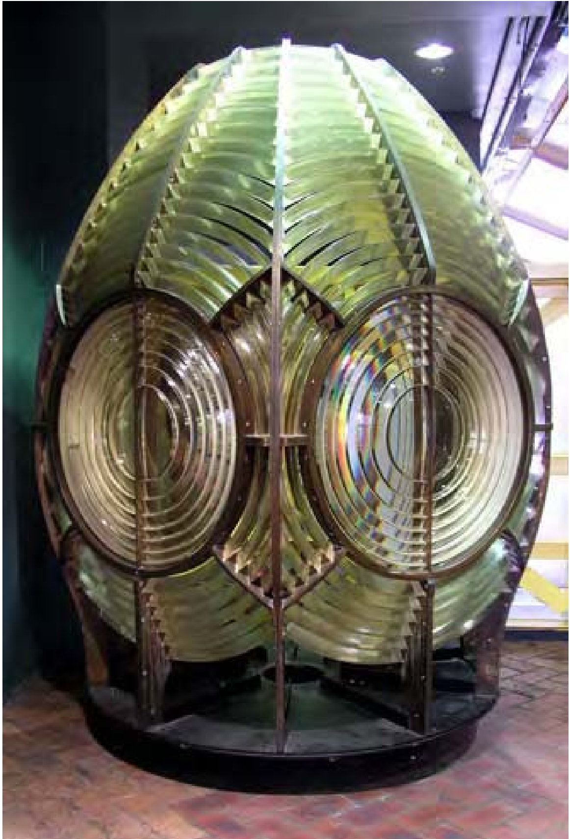
Figure 23 – A Fresnel lens from the Dog Island Lighthouse formally on display at the Museum of City and Sea in Wellington.
