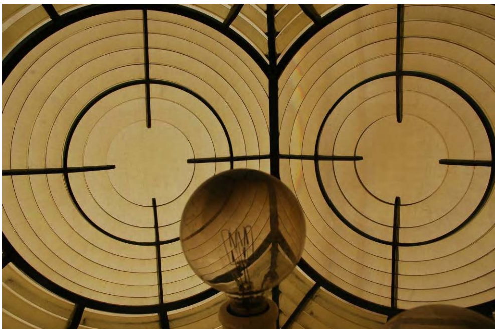
Figure 21 – The two ‘bulls eyes’ in the Cape Brett lens.
