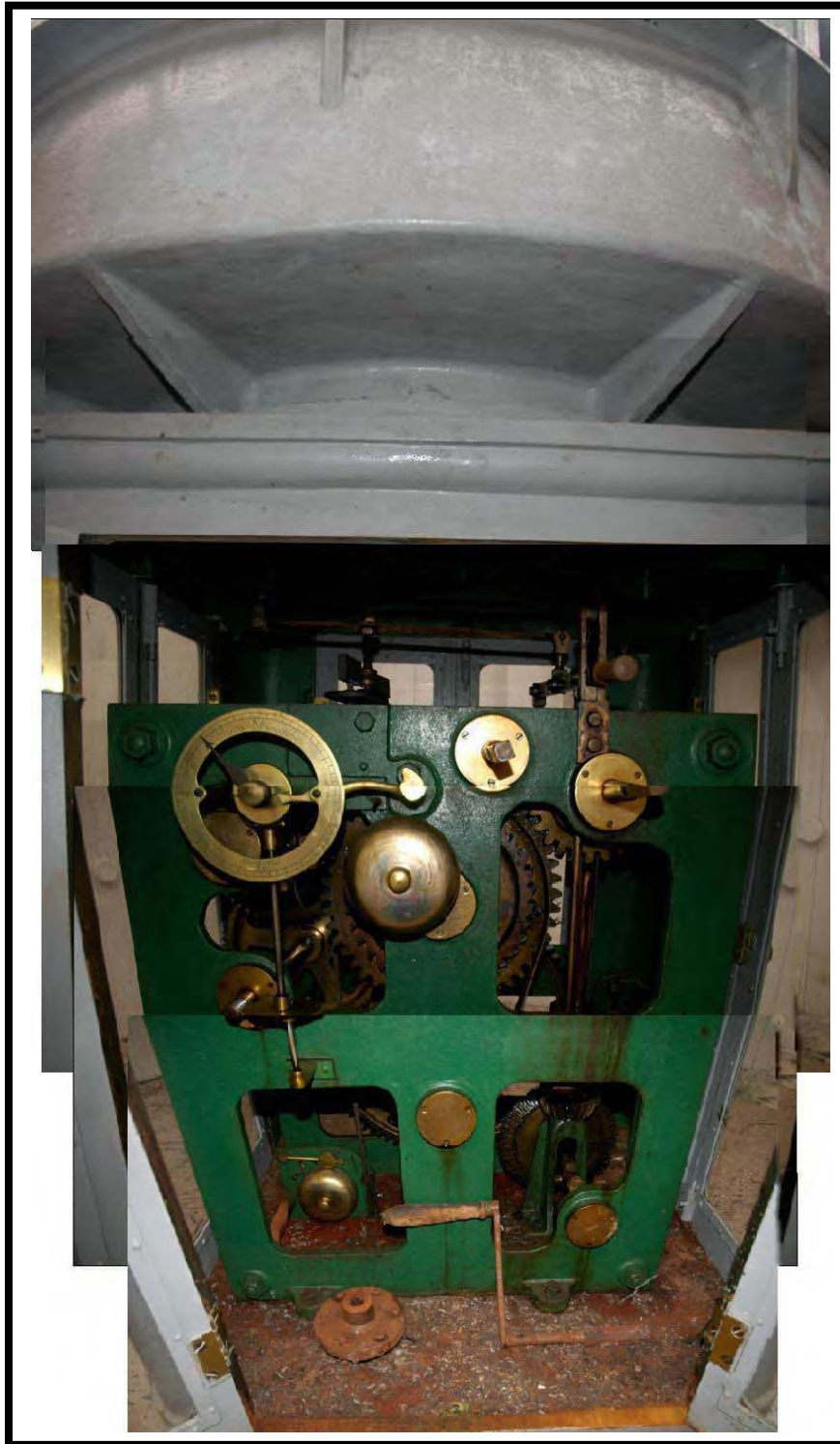
Figure 31 – The mechanism that sits beneath the mercury bath.
