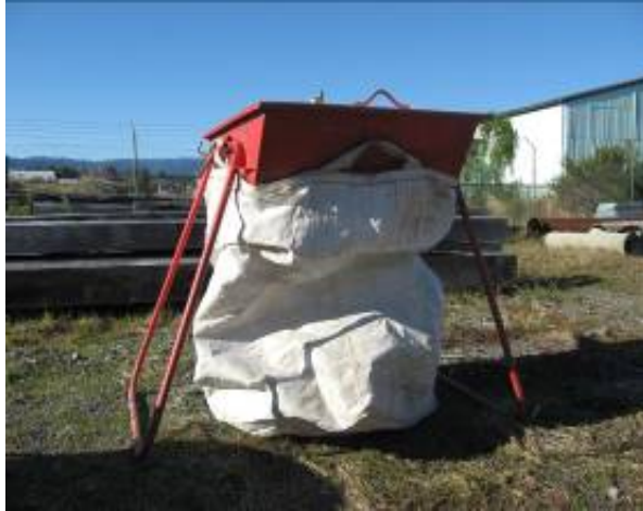
Figure 64 – Loading frame designed to be loaded by either a tractor or digger
