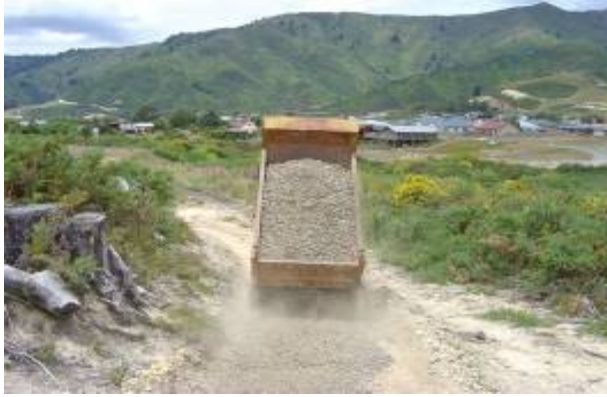
Figure 62 – Modern power carriers have a hydraulic tilt function making the spreading of material significantly easier
