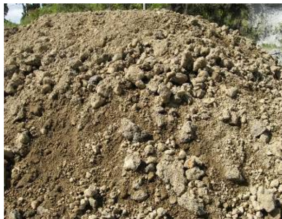
Figure 46- Stockpile of poorly graded material ready to be used as a track surface
