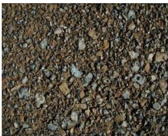
Figure 48b - A well graded metal track surface. Note the stones are angular and there is a good distribution of particle sizes. The presence of fines “locks the material together”. Particle sizes vary from 20 mm to 0.002 mm
