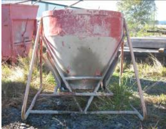
Figure 66 – Hoppers are available in a few different shapes and sizes. This hopper consists of a cylinder on the top and a truncated cone on the lower portion
