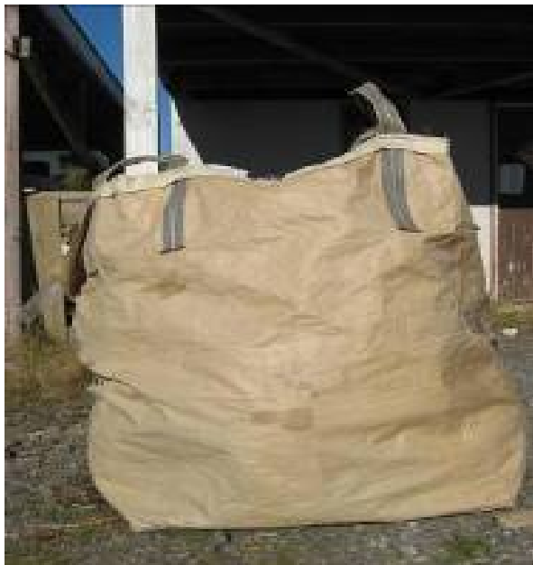
Figures 63 – Fadges are cheap and available in a number of different sizes. They can be pre-filled with material several days prior to flying
