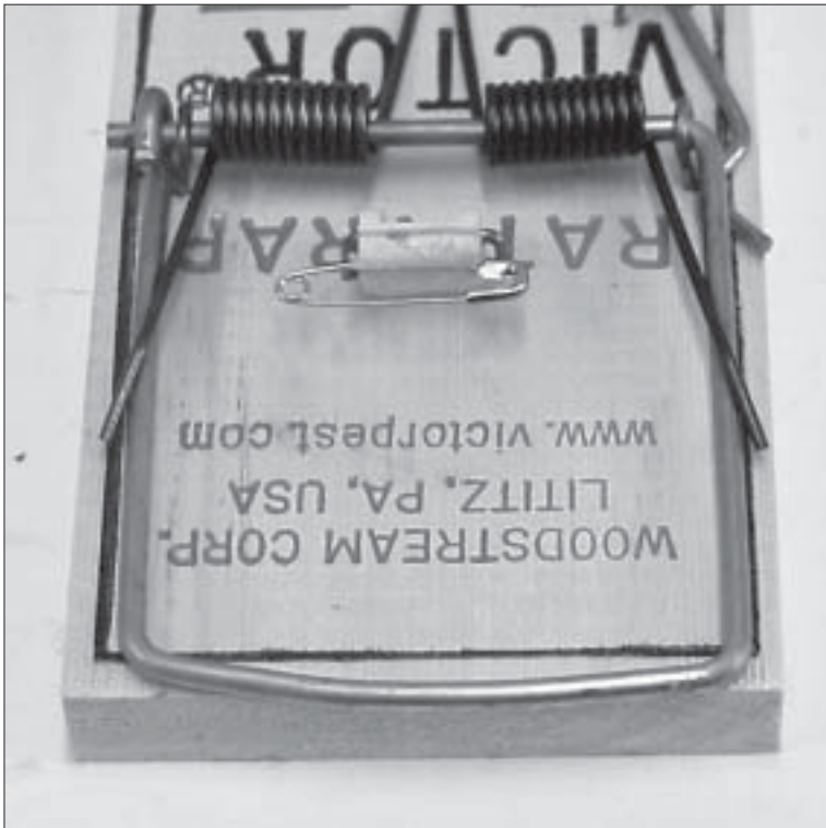
Figure 2. Trap with plastic trigger base and safety pin attached.
