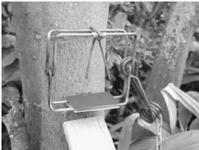
Figure 1. The SA Conibear kill-trap set in a metal bracket as supplied by DOC. A small pile of mince or tinned cat food is placed on top of the bracket (not shown), and when the cat feeds on the bait, the top of the cat's head triggers the trap.
