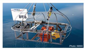
Special equipment is needed to survey the deep seabed. DTIS is equipped with high-definition video and still cameras, floodlights and a depth sensor. Towed behind a research vessel, DTIS relays a live stream of underwater footage to the vessel above.
