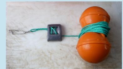
Modified floats consisted of two 150 mm floats on 4 fathom (7.2) m ropes (unless stated otherwise), with a 1.3 kg lead weight at the clip.
