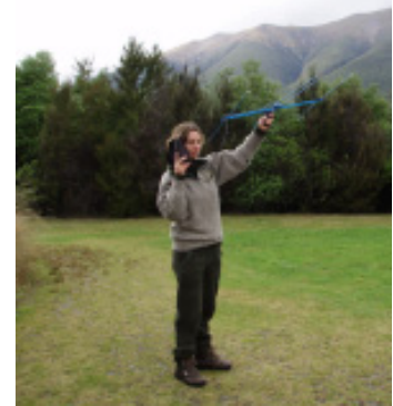
RNRP Ranger Tamsin Bruce radio tracking kaka. The radio transmitters attached to the kaka are able to be tracked using telemetry.
