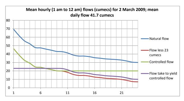
Figure 1. Modelling of possible controlled flows in the Morgan Gorge producing flows suitable for kayaking on days where the natural flows are too high
