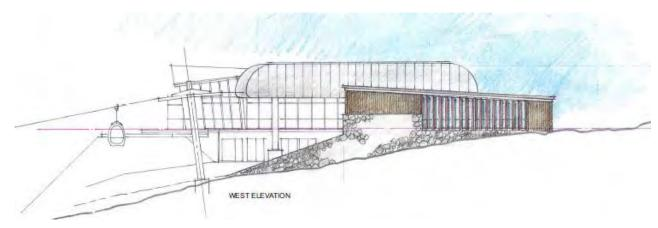
Image 15 - Upper terminal west elevation showing architecturally designed building in foreground (coloured) with proposed gondola terminal structure (grey) behind and existing Knoll Ridge Café (line sketch) at rear
