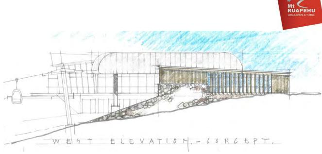
Image 2 - Upper terminal west elevation, existing Knoll Ridge Café shown behind in black and white
