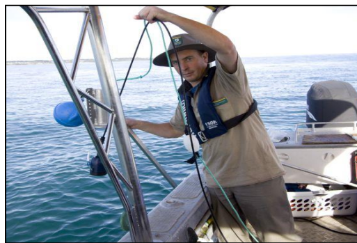
Figure 27. Immediately prior to deployment. Note: The BUV coaxial cord (black) plus surface rope (green) and buoy (not in field of view) are held together by the surveyor to reduce the chance of entanglement.
