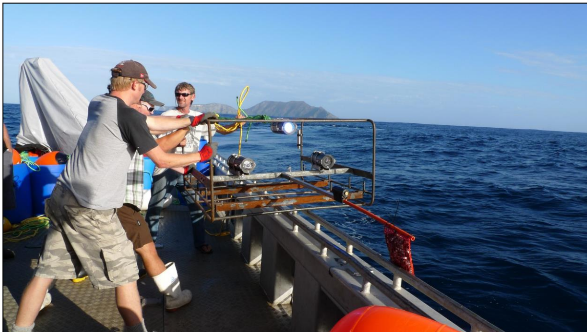
Figure 2. Forward-facing BUV system deployed by Te Papa scientists off the Three Kings Islands. Note the heavyweight bars at the base of the unit, the two video housings for the stereo system, which allows for measurement in three dimensions, and the lighting system. This unit is set up to be sent to 1200 m. Similar but lighter units are used at shallower depths.
