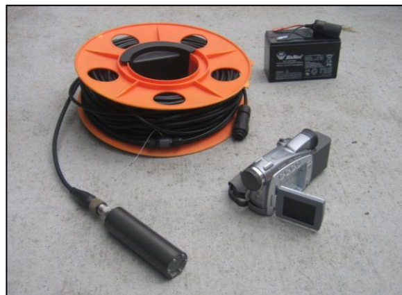
Figure 22. Drop camera equipment: (A) MDEL drop camera and 70 m coaxial cable; (B) 12 V rechargeable battery pack used to power the drop camera unit; and (C) digital video recorder with movable screen. This setup is used for real time substratum and habitat assessment. All components are linked together in a customised waterproof case (not shown). Note: The video recorder is powered by a long-life (8 h) 7.4 V battery pack specific to the video recorder.
