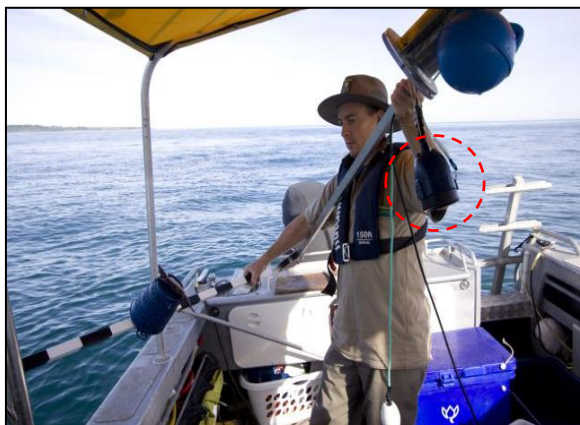
Figure 21. BUV setup prior to deployment. Red circle denotes Splashcam® drop camera. The drop camera is in this case used to assess habitat suitability at the start of the deployment. If providing good image quality, the drop camera can also be directly used to record the video data, effectively replacing the video camera in its housing.
