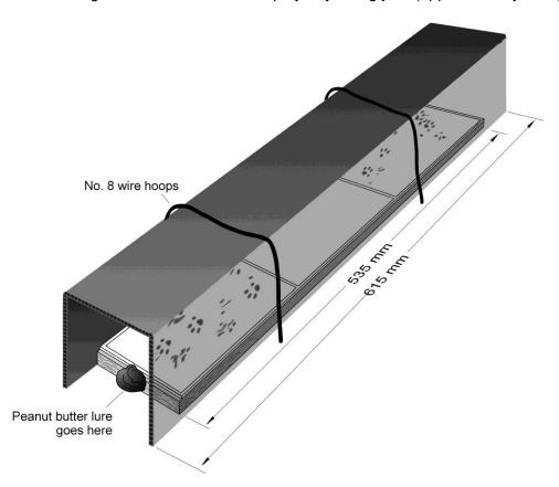
Figure 1. Black corflute tracking tunnel cover and wooden base, showing tunnel dimensions. Also shown is the location for smearing peanut butter on the vertical face of the wooden base at each end of the tunnel for rodent surveys.
