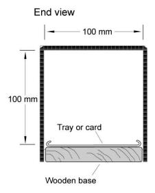
Figure 2. Black corflute tracking tunnel cover and wooden base—end view showing tunnel dimensions.
