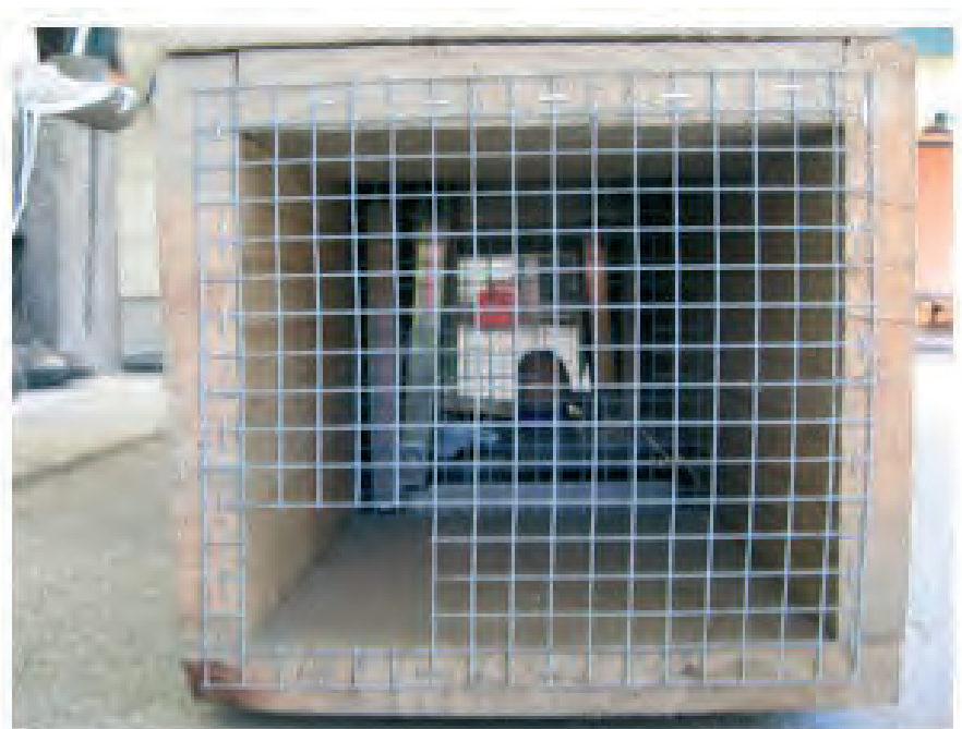
Figure 2.3f DOC 200 double sets – external baffle set up in a box (offset)
