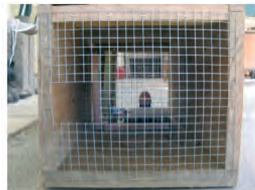
Figure 3.1f DOC 250 single set – external baffle set up in a box (offset)
