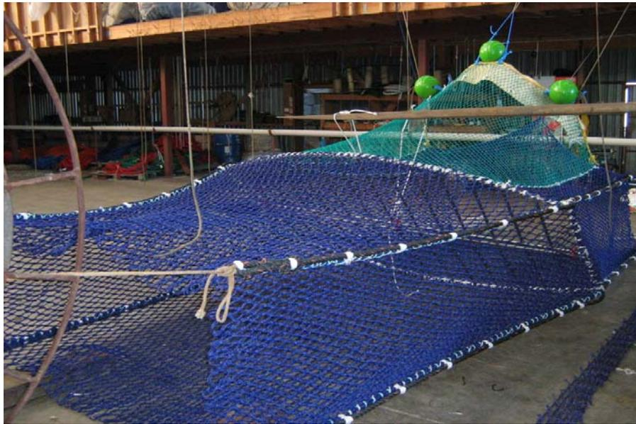
**Figure 16:** SED viewed from behind, final lengthener and codends attach at end closest to observer.
