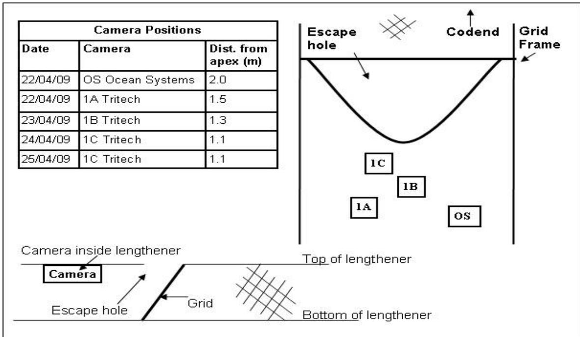
**Figure 6:** Camera placements for second sea trials, side and plan views. Note OS camera failed after two tows.
