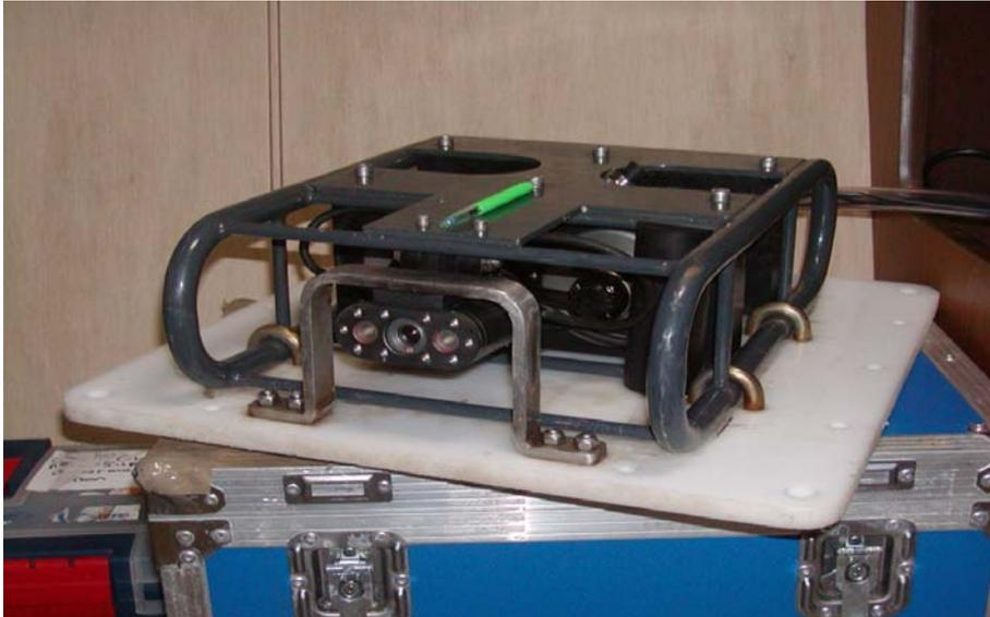
**Figure 5:** Trittech Seacorder white light camera. The Teflon base board and stainless protection bar were added to improve usability and protection. Ball point pen lying on top provides scale.
