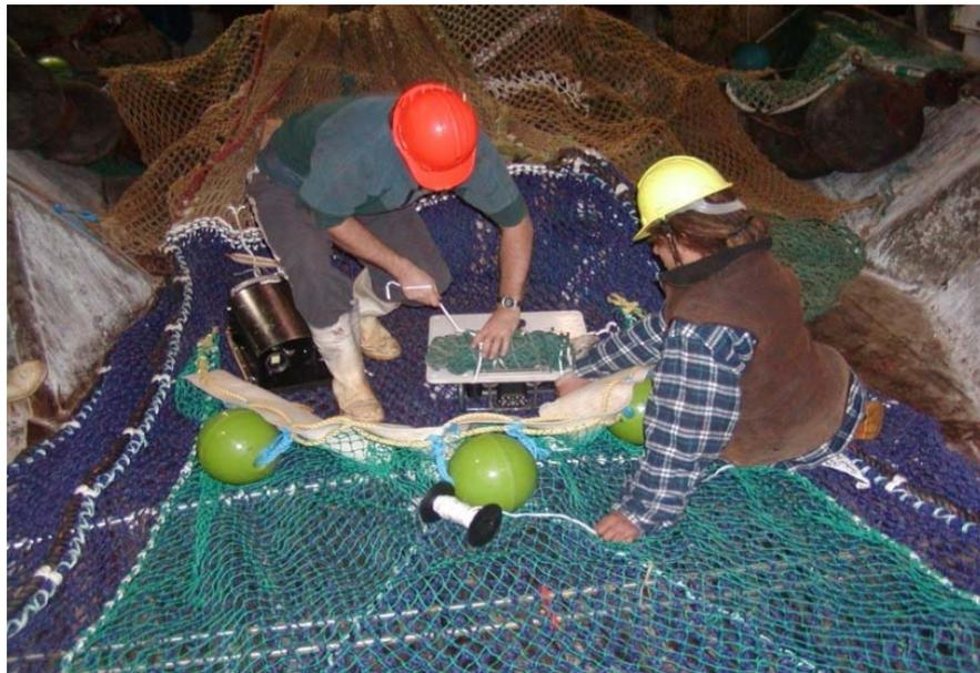
**Figure 1:** Deck crew fitting the cameras to the SED with netting packing to improve field of view, *FV Taimania*, April 2009
