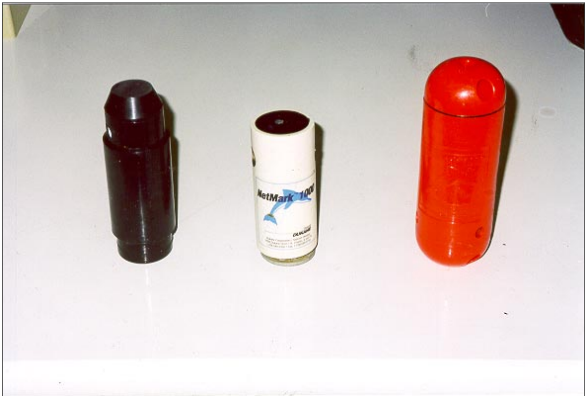
Figure 2. Photograph of the pingers used in this experiment. The red DUKANE® and black PICE® are both commercially available pingers, and the white DUKANE® is an experimental model developed by the company as a prototype in 1994.
