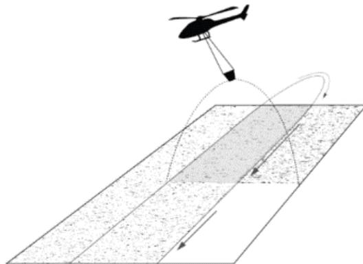
Figure 12. Bait-spreading pattern illustrating 50% overlap of bait swaths (Broome et al. 2017)
