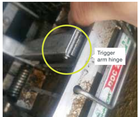
Figure 6. Aerial view of hinge connecting trigger arm to trigger hanger.
