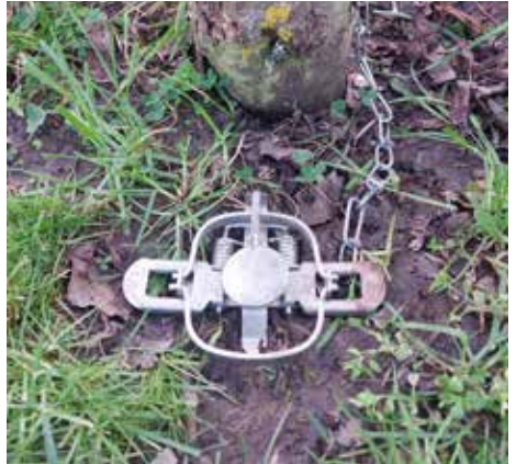
Victor No.1 double coil spring unpadding, used in live capture possum trapping. Photo: Tim Sjoberg
