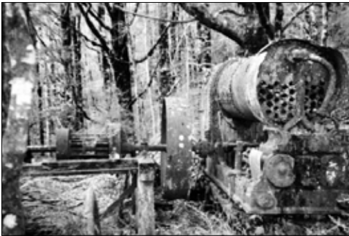
Figure 8. The patent Robey fixed engine.
