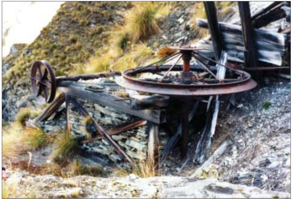
Figure 33. The All Nations aerial cableway top return wheel. Note the similarity to the Homeward Bound wheel (Fig. 20). Photo: P. Petchey.
