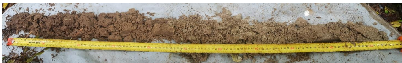
Figure 10. Soil/subsoil profile showing loosely consolidated quartzose sediments down to at least metre in depth (i.e. tape length shown).
