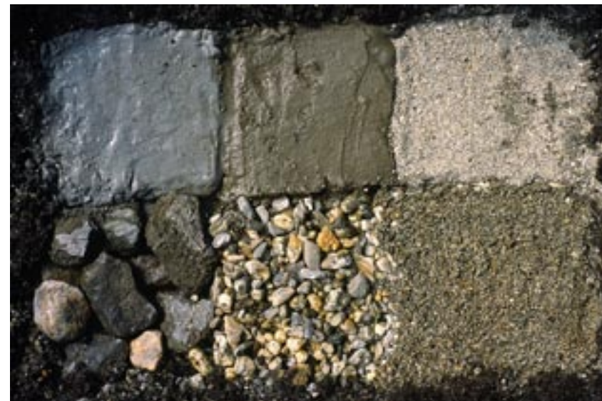
Fig. 130 An example of particle sizes, clockwise from top left: fine silt, silt, sand, coarse sand, gravel, coarse gravel. These are from a bay head at Lake Wanaka, Otago. Each square of material is 15 × 15 cm. The fine silt (top left) is dense and plastic, being originally glacial flour that settled on the bed of a former ice-snout lake. The silt at top centre is brownish from being partly weathered, and because it includes some humus material. The materials had been sorted to their respective particle sizes by the differential energies of wave action. Particle size of inorganic materials influences the drainage characteristics and fertility of many lacustrine, riverine, and estuarine wetlands. Many peatlands are underlain by one or more of these types of material.
