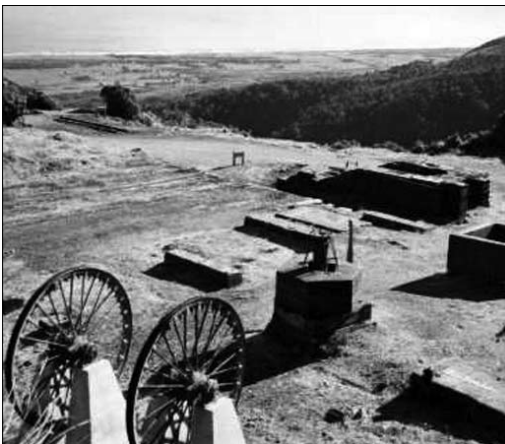
Figure 9. Cable wheels, located near the top of the Denniston Incline, West Coast.
