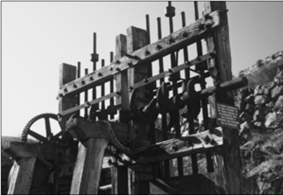
Figure 1. Stamper battery, Bendigo Reserve, Otago.
