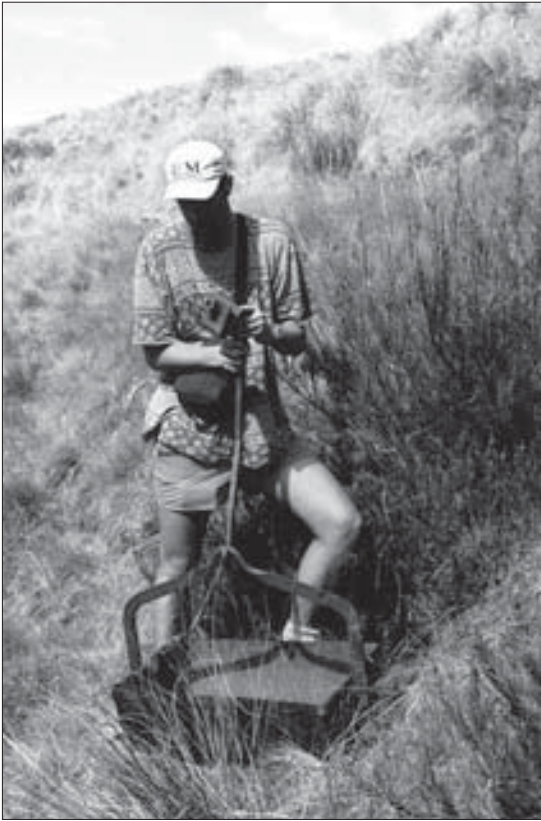
Figure 10. British-American Spur cableway ore bucket and hook assembly (held by A. Braden). Photo: P. Petchey.
